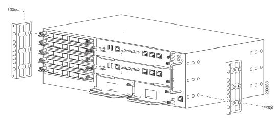
Figure 3-2 shows how to attach the brackets on the Cisco ASR 903 Router for a 300 mm ETSI cabinet.
